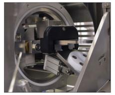
Optional handle maker consistently produces a correctly-sized loop with no wasted netting.
