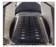
Optional roller belt inside horn assists products through the chute.
