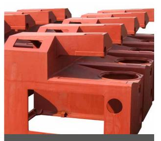
A separate cast-iron base is developed for each cutter size. Together with the solid rust-free outer surfaces, it is the perfect basis for a highly resilient and highly efficient machine.
