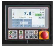
Innovative touch panel with a clean user interface design. All the important settings, such as knife and bowl speeds, switch-off functions, etc. can be freely configured.
