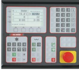
Bowl cutter 33 L, type 425. Operation via foil keyboard (T2). Knife shaft and bowl can be driven at two speeds
